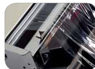
1. Profilo teflonato Teflon-coated section
