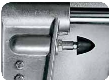
11. Paracolpo carrello Hopper's buffer
